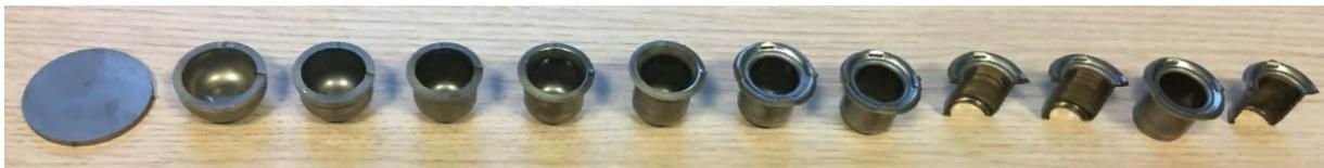
Figure 3: Cup after the different phases of the production process.
