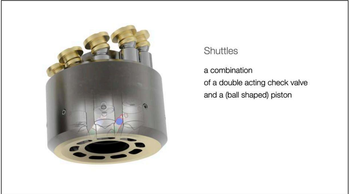
Shuttles act as check valves when the ball is pressed into one of the two seats. But the ball also acts as a small piston, when it is moving from one seat to the other.
