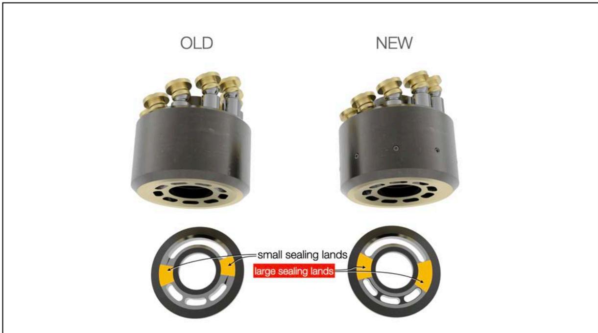
The second change is that we increased the size of the sealing lands. When a barrel port is blocked by the sealing land, there is no connection to either the low or high pressure side of the pump. As a result, the oil in the cylinder will be compressed or expanded due the piston movement and the blocked barrel port.
