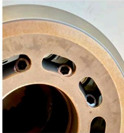
Shuttles are not a general solution for all pumps and motors. So far, we only tested the shuttles in a 28 cc slipper type pump and a 45 cc floating cup pump.
