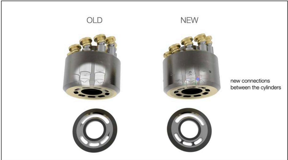
The third change is not in the valve plate, but in the barrel. We made new connections between the cylinders inside the barrel. We call these connections shuttles.
